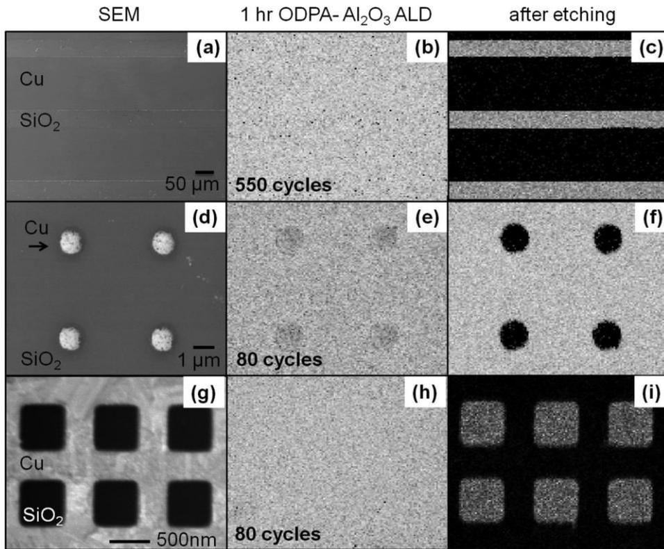
**Figure 1.** Demonstration of 2-D area selectivity. (a, d, g) Scanning electron microscopy images of patterned Cu/SiO<sub>2</sub> substrates. (b, e, h) Al Auger map of the patterned Cu/SiO<sub>2</sub> substrates treated with octadecylphosphonic acid for 1 h and (b) 250, (e) and (h) 80 cycles of Al<sub>2</sub>O<sub>3</sub> ALD. (c, f, i) Al Auger map after the self-correcting etch process is carried out. Figure from Reference [2].
