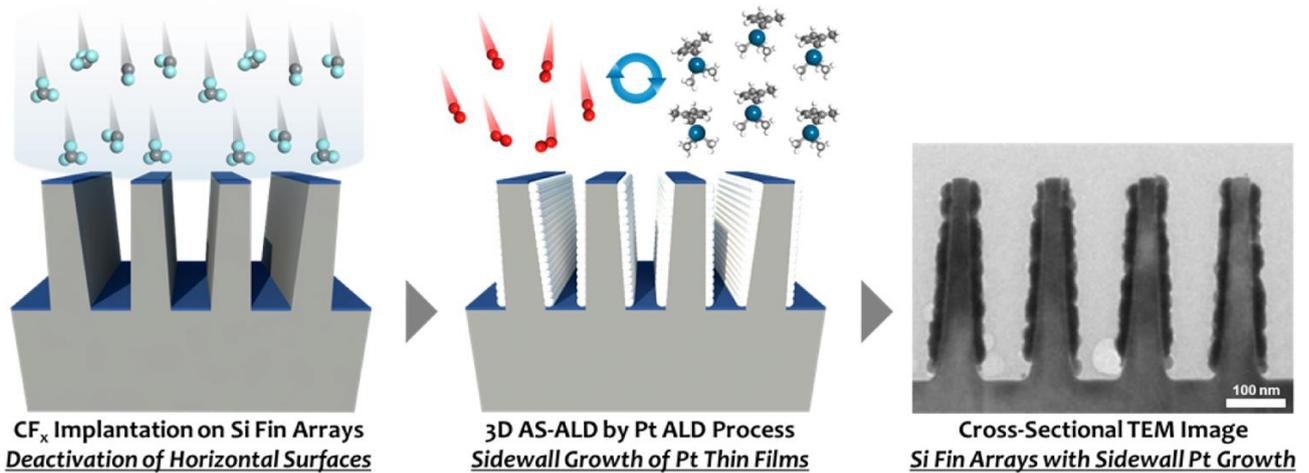
**Figure 2.** (Left and Center) Schematic of the topographically selective ALD process. (Right) Cross sectional TEM image of a silicon fin array substrate after the process, showing topographical selectivity in which Pt is deposited only on the vertical sidewalls after the horizontal surfaces are blocked by CF<sub>x</sub> implantation. Figure from Reference [3].
