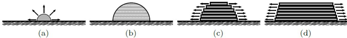
**Figure 3.** Schematic representation of nucleation mechanism of SnS<sub>2</sub> or SnS CVD: (a) initial nucleation of amorphous island, (b) crystallization of initial island at critical dimension, (c, d) preferential horizontal growth due to a higher reactivity of the crystal edges as compared to the horizontally arranged basal planes.
