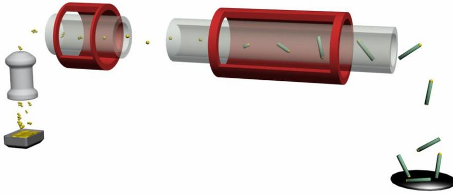
**Figure 1.** Principle of nanowire growth by aerotaxy, going from left to right: Au is evaporated, forming an aerosol of Au particles, which are size-selected, sintered, mixed with  $\text{AsH}_3$  and TMGa in a tube furnace, and collected on a substrate. In this continuous flow process,  $10^9$  particles per second grow into nanowires at a rate of around  $1 \mu\text{m/s}$  [5].
