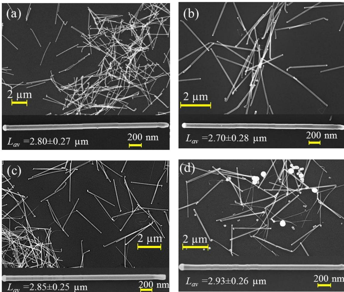
**Figure 2.** SEM images of  $\text{GaAs}_{(1-x)}\text{P}_x$  NWs grown at  $550^\circ\text{C}$  and with  $x =$  (a) 0.00 [pure GaAs] (b) 0.25, (c) 0.50 and (d) 0.75.  $L_{av}$  represents the average NW length with the  $\pm$  fractions representing one standard deviation based on 30 measured wires. The lower panel in each image is a representative single NW image [7].
